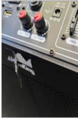
False Nameplate Peeling Off
